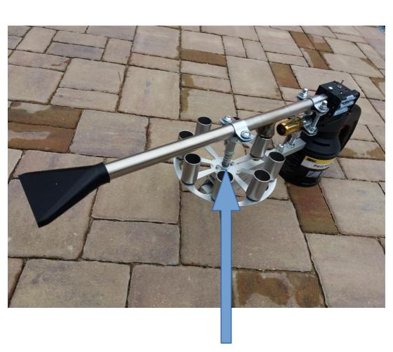
Once a season put a drop of high temperature resistant lubricant into the center of the carousel to lubricate the plain bearing.
